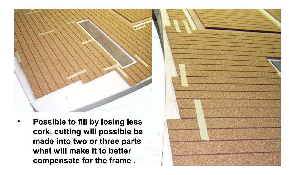
Well on, to maintain in place all the parts, the adhesive of masking is essential.
