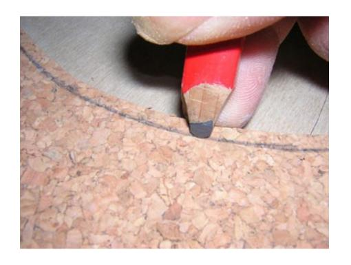
After cutting of the plank you traces then the width of the groove (4 mm) with attention not to be been mistaken in with dimensions.
